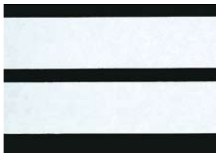
Tape test with SEFAR® PET 1500: The absence of stencil residue on the adhesive strips is proof of SEFAR® PET 1500's excellent adhesion characteristics
