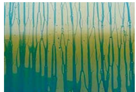
Untreated high-modulus mesh: nonuniform wetting
