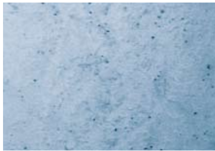
Ink deposit with SEFAR® PET 1500: The picture shows the more uniform ink deposit with SEFAR® PET 1500
