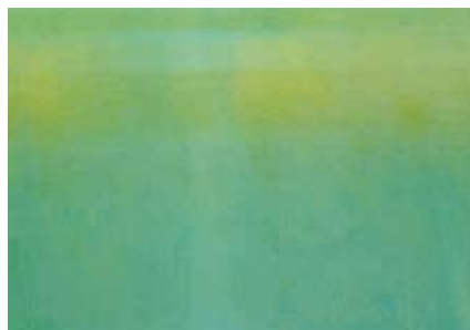
SEFAR® PET 1500 – uniform wetting: A test with dyed water clearly reveals the difference in wetting characteristics
